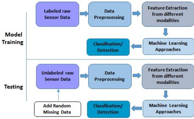
Fig 1. Flow diagram for sensor-based activity recognition considering missing data patterns.
